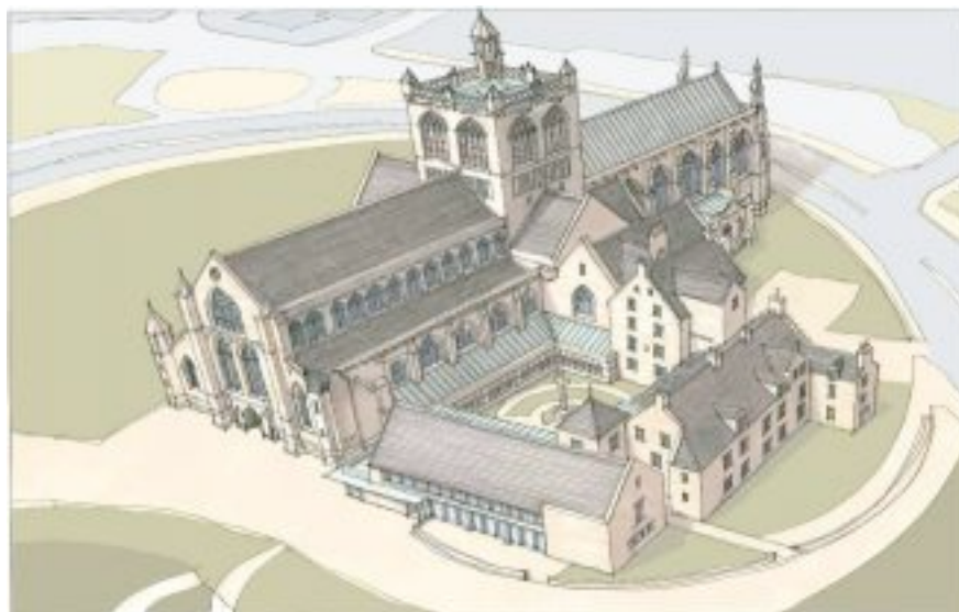
Figure 3: Proposal to re-enclose the cloister garth of Paisley Abbey with a new building shown at the bottom of the picture
